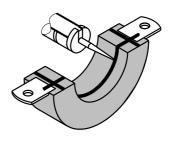
Type 173 F At the factory-premounted construction only the upper part may be removed. Then the halfs are sealed with dipa® seal paste Type 4045 (Item No. 31004966, catalogue page 174) as Type 170. The steel brackets, which connect through the middle thread with the low temperature clamps, are not allowed to be dissembled.
